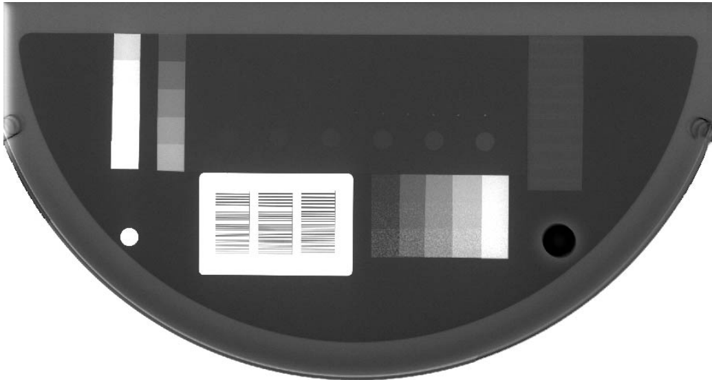
Figure 6: Leeds TOR MAS phantom groups several test objects for measuring low and high contrast, spatial resolution, details and masses (from Leeds Test Objects).
